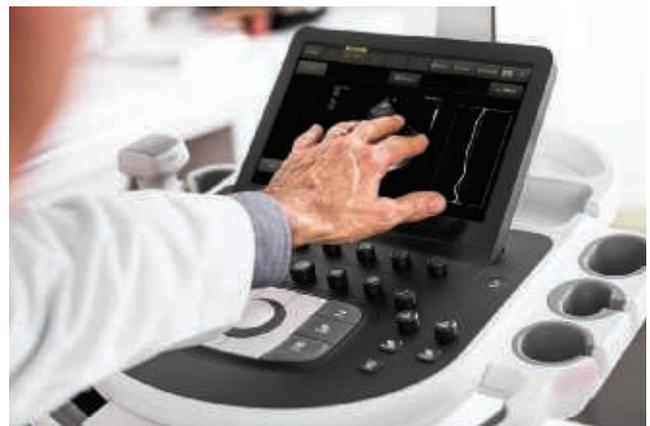
**With image replication and TGCs on its tablet touchscreen, Affiniti 30 was designed to reduce reach and button pushes.**
